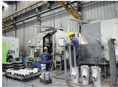
CNC Boring Machine
